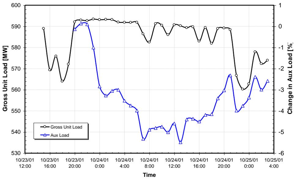
Figure 10: Reduction in Auxiliary Power Measured During the Second Coal Burn Test
