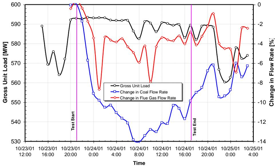
Figure 7: Variation of Coal and Flue Gas Flow Rates During the Second Coal Burn Test
