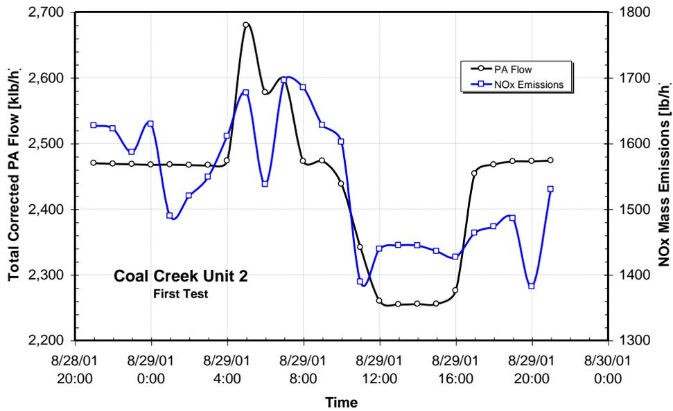
Figure 13: Variation in PA Flow and Mass Emissions of NO<sub>x</sub> During the First Coal Burn Test
