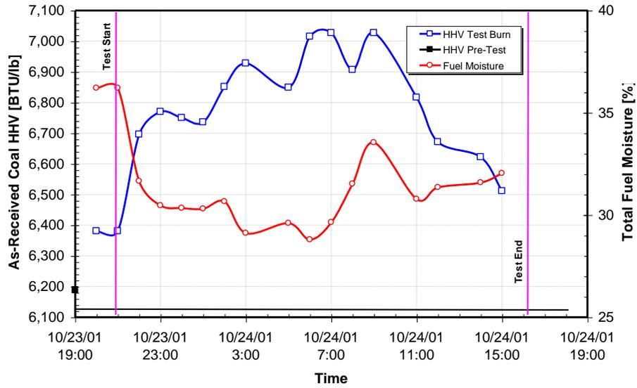
Figure 6: Variation of Coal HHV and Moisture Content During the Second Coal Burn Test
