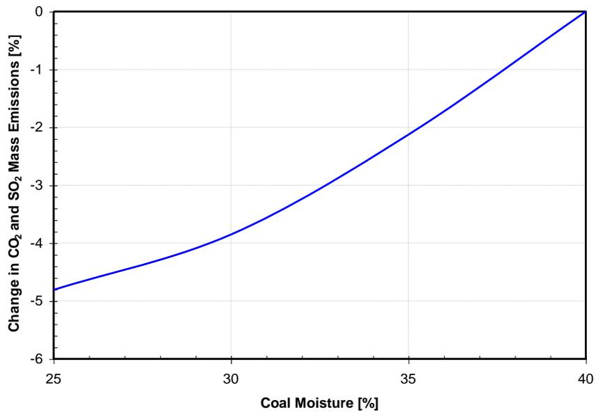
Figure 5: Effect of Coal Moisture on Mass Emissions of CO<sub>2</sub> and SO<sub>2</sub>
