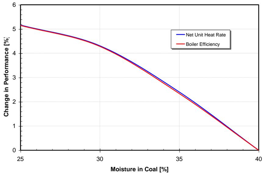
Figure 3: Effect of Coal Moisture on Boiler and Unit Performance
