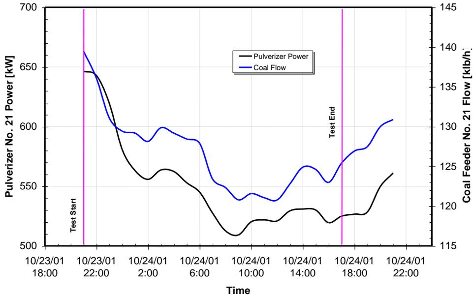
Figure 9: Variation of Pulverizer Power and Pulverizer Coal Flow During the Second Coal Burn Test for No. 21 Pulverizer
