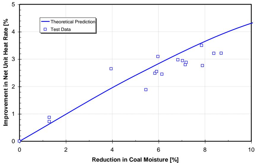
Figure 11: Improvement in Net Unit Heat Rate Versus the Reduction in Coal Moisture Content
