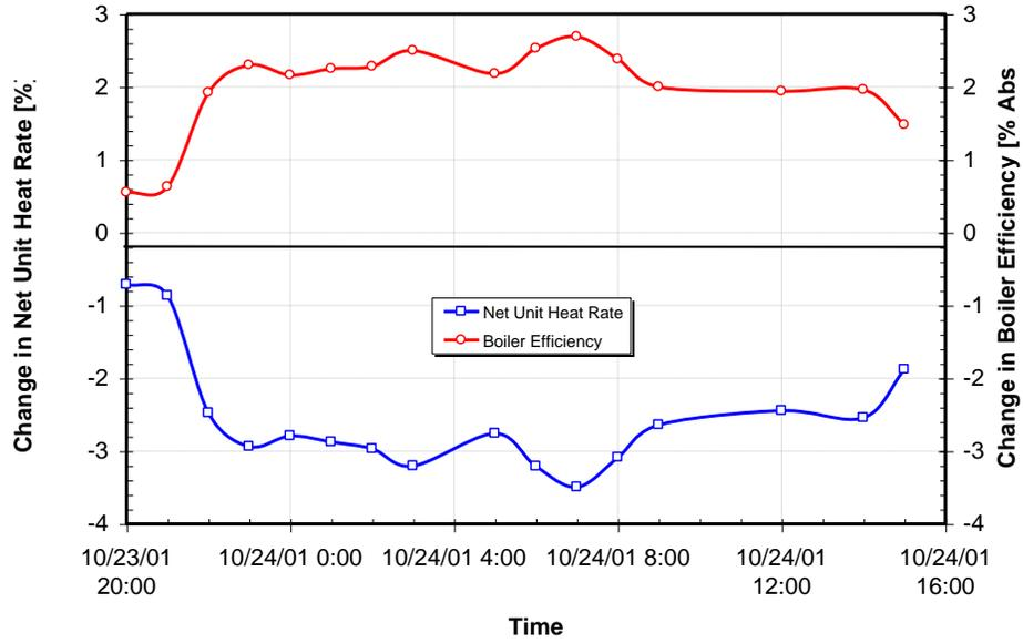
Figure 12: Variation of Boiler Efficiency and Net Unit Heat Rate During the Second Coal Burn Test
