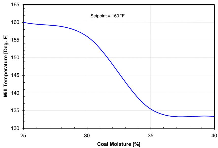
Figure 4: Effect of Coal Moisture on Mill Temperature
